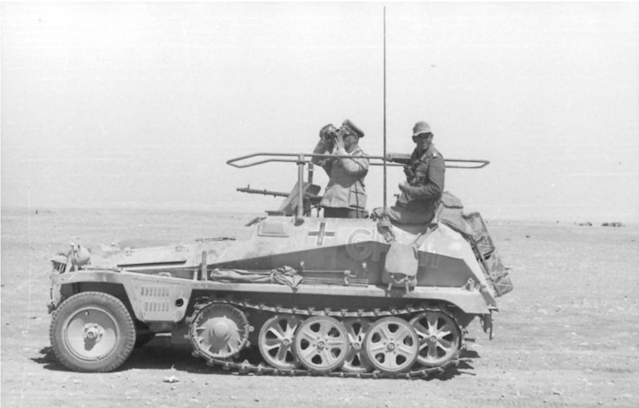
Fig. 1.13 Erwin Rommel (with binoculars) in his Sd.Kfz 250/3 half-track ‘Greif’ during the African campaigns. Half-tracks are a useful compromise vehicle for difficult terrain, balancing traction and manoeuvrability. Bundesarchiv—Wikimedia Commons
