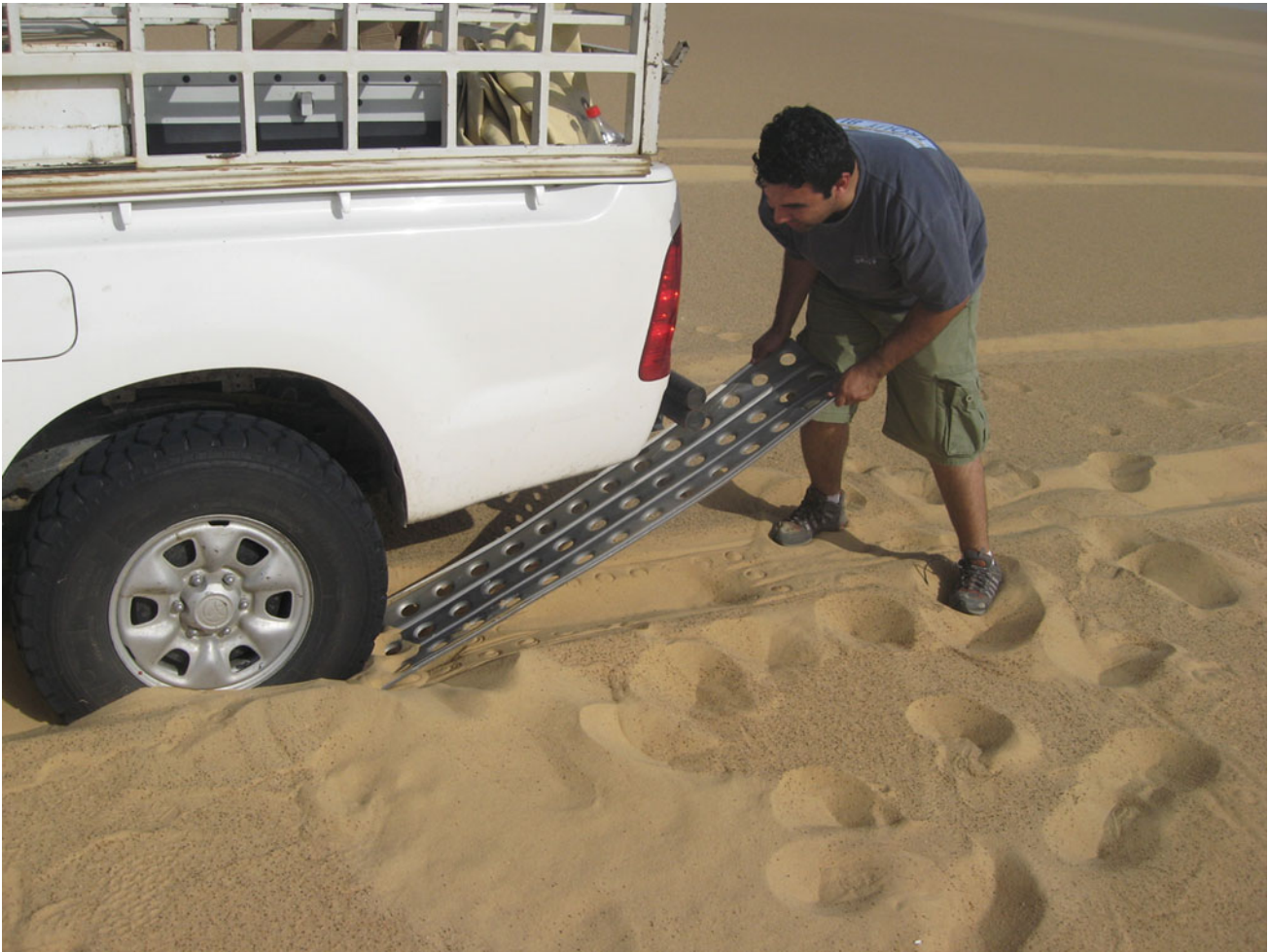
Fig. 22.10 JPL scientist Essam Heggy, during a ground-penetrating radar measurement campaign in Egypt, shoving a perforated sand channel under the tire of a vehicle stuck in sand in preparation for backing out after getting stuck in soft sand moving uphill—sometimes it is easier to go back than forward. Photo Ralph Lorenz
