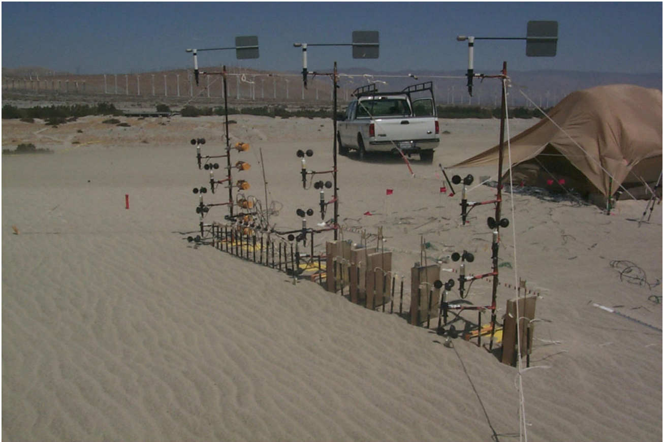
Fig. 16.13 A modern field experiment can be an orgy of instrumentation. Here we see an array of sand traps ( boxes ), safire detectors (narrow cylinders in the ground), cup anemometers and wind vanes. The data acquisition equipment is prudently protected in a tent (the shade in
