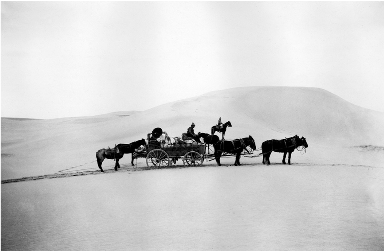
Fig. 22.3 Where camels are unavailable, explorers made do with horses. This early US Geological Survey team struggles across a dune in Wyoming in 1907. Note that the narrow wheels on this wagon are poorly-designed for soft sand, and have sunk in appreciably. Photo USGS
