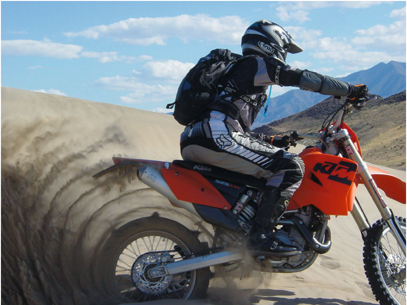
Fig. 22.7 Sheets of sand being thrown up by the bike's rear paddle tire—note the ridges at 45° intervals. While these provide powerful traction on loose dune sands, they would be unpleasant and unsafe for road use. Photo by Kevin Rice, Wikipedia/Creative Commons License
