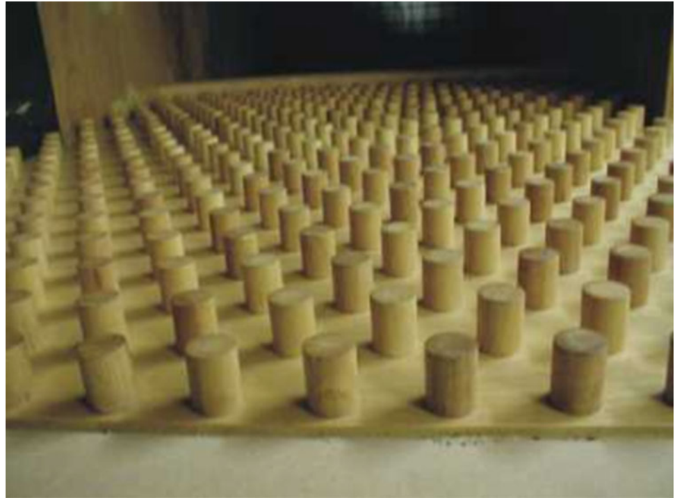
Fig. 17.7 An arrangement of roughness elements designed to control the thickness of the boundary layer (see Sect. 4.2) in the Trent tunnel
