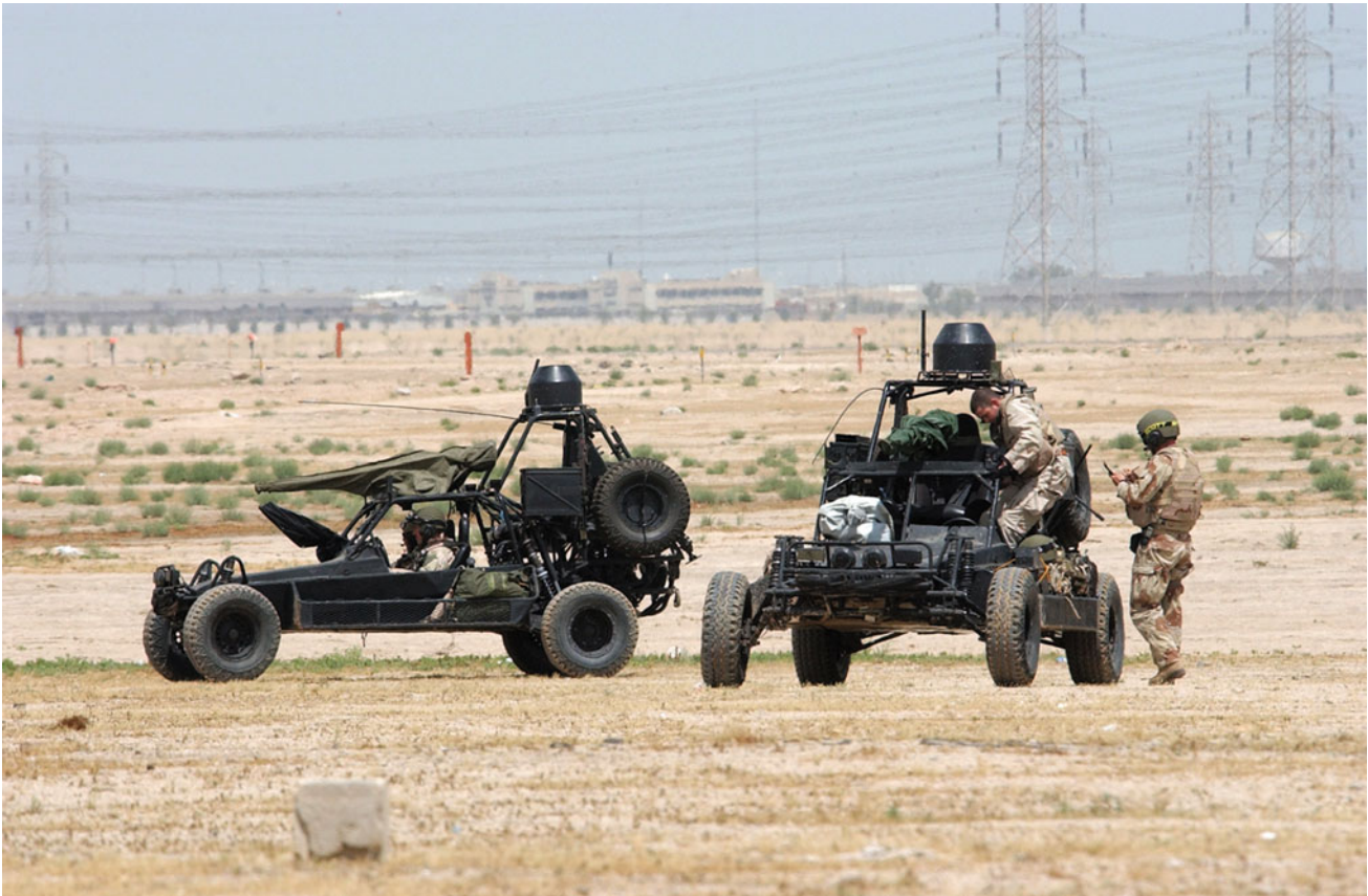
Fig. 22.6 Military dune buggies. These are Desert Patrol Vehicles (DPVs) operated by the US Navy Seals, that permit high speed driving in desert terrain for special operations. Note the low center of gravity,
