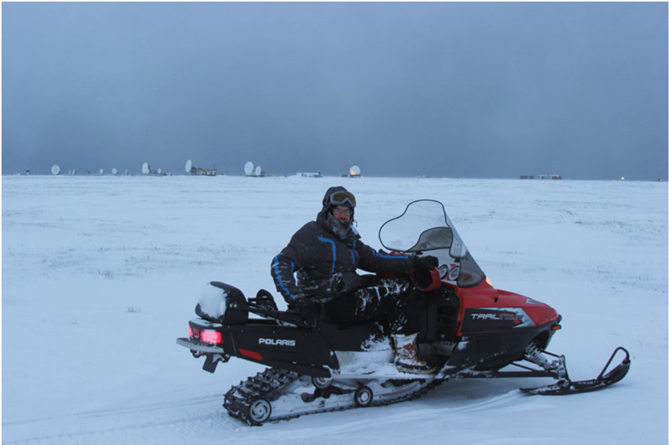
Fig. 22.4 Hybrid vehicles such as half-tracks or here, a snowmobile, are useful compromises between the low ground loading and superior traction of a long track at the rear and independently-movable steering
