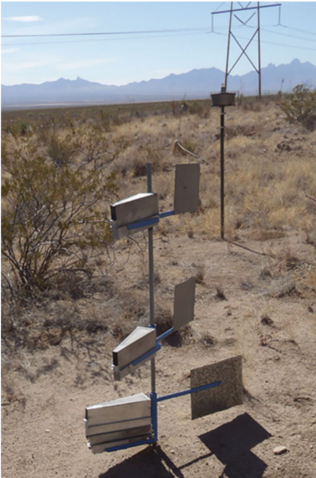
Fig. 21.1 Sand trap at La Jornada Experimental Range, New Mexico, used to evaluate the agricultural impact of aeolian processes. This simple but effective vane/pivot arrangement points three flared two-part boxes upwind at different height: the triangular flare decelerates the air, which escapes through a wire mesh at top while the sand collects in the closed bin. After some sampling period (usually weeks) the boxes are opened and the time-integral soil transport is evaluated by weighing. Photo R. Lorenz
