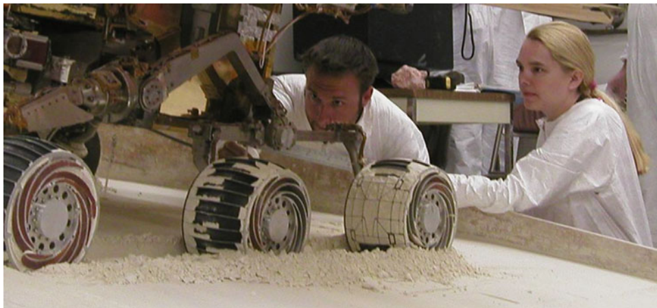
Fig. 1.14 Mike Seibert and Sharon Laubach, engineers on the Mars Exploration Rover team at NASA’s Jet Propulsion Laboratory, Pasadena, check the exact position of a test rover in preparation for the next test of a possible maneuver for Spirit to use on Mars. The test setup at JPL simulates the situation where Spirit is embedded in a patch of soft soil dubbed ‘Troy’, in Mars’ Gusev Crater. The preparation shown here on July 7, 2009, preceded an assessment of straight-backward driving the next day, one of several possible maneuvers assessed in the test sandbox. Image Credit NASA/JPL-Caltech
