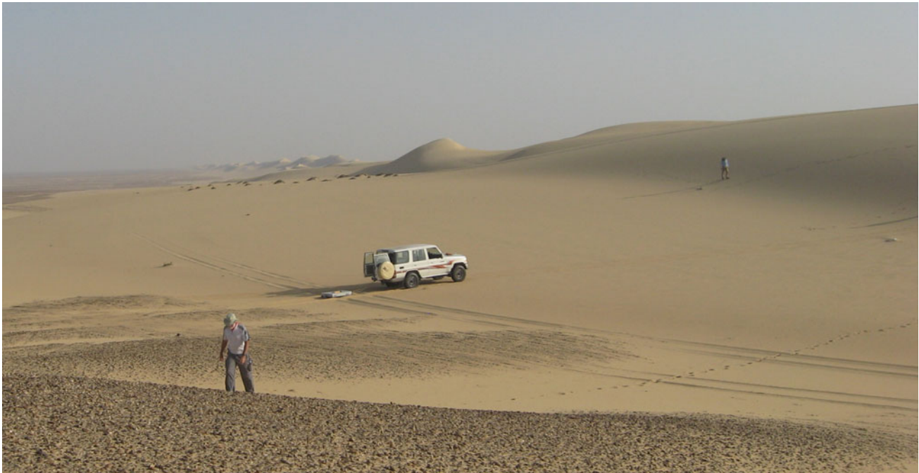
Fig. 16.12 Using a vehicle to drag a GPR system across a linear dune at Quattaniya, Egypt. Note this GPR is a longer wavelength antenna than that shown in Fig. 16.8 and thus is physically rather larger. Photo R. Lorenz
