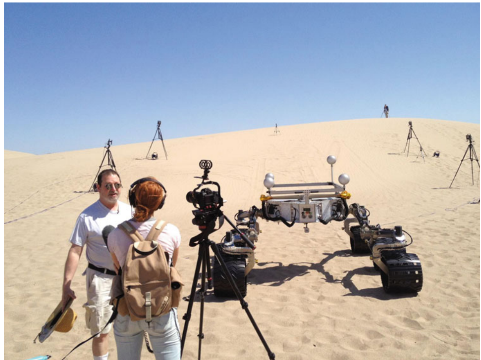
Fig. 22.15 Michael Malin, left , a prominent Mars scientist, comments to a news reporter during tests of the ‘Scarecrow’ rover on Dumont Dunes in California’s Mojave Desert in May 2012 to determine its performance in driving up various slopes on windward and downwind portions of dunes. This is a stripped-down mobility test rover, designed to have the same weight on Earth as the full Curiosity rover has on Mars. Image credit NASA/JPL-Caltech
