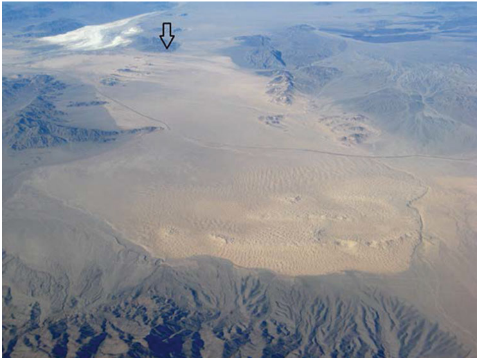
Fig. 8.3 An example of a regional sand transport system, viewed from an airliner. The Kelso dunes in southern California are seen at the bottom of the picture, looking north: the sand accumulates in part due to topographic blocking and in part due to convergent winds. A dominant pathway for the sand (sourced primarily from the Mojave
