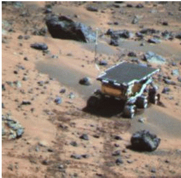
Fig. 16.21 The Sojourner rover imaged by the Pathfinder lander in 1997. The rover has stopped atop a shallow ripple, nicknamed 'Mermaid', where it used an APXS instrument to measure the sand composition. NASA/JPL/U.Arizona
