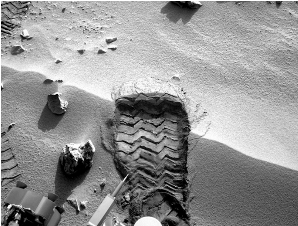
Fig. 16.20 Mars exploration rover wheel tread on a ripple. Note the 'bulldozed' lobe of material, the crisp imprint of the rover wheel tread pattern, the steep walls of the 'trench' and the radial fractures in the material indicating some cohesion. NASA/JPL PIA 1620543
