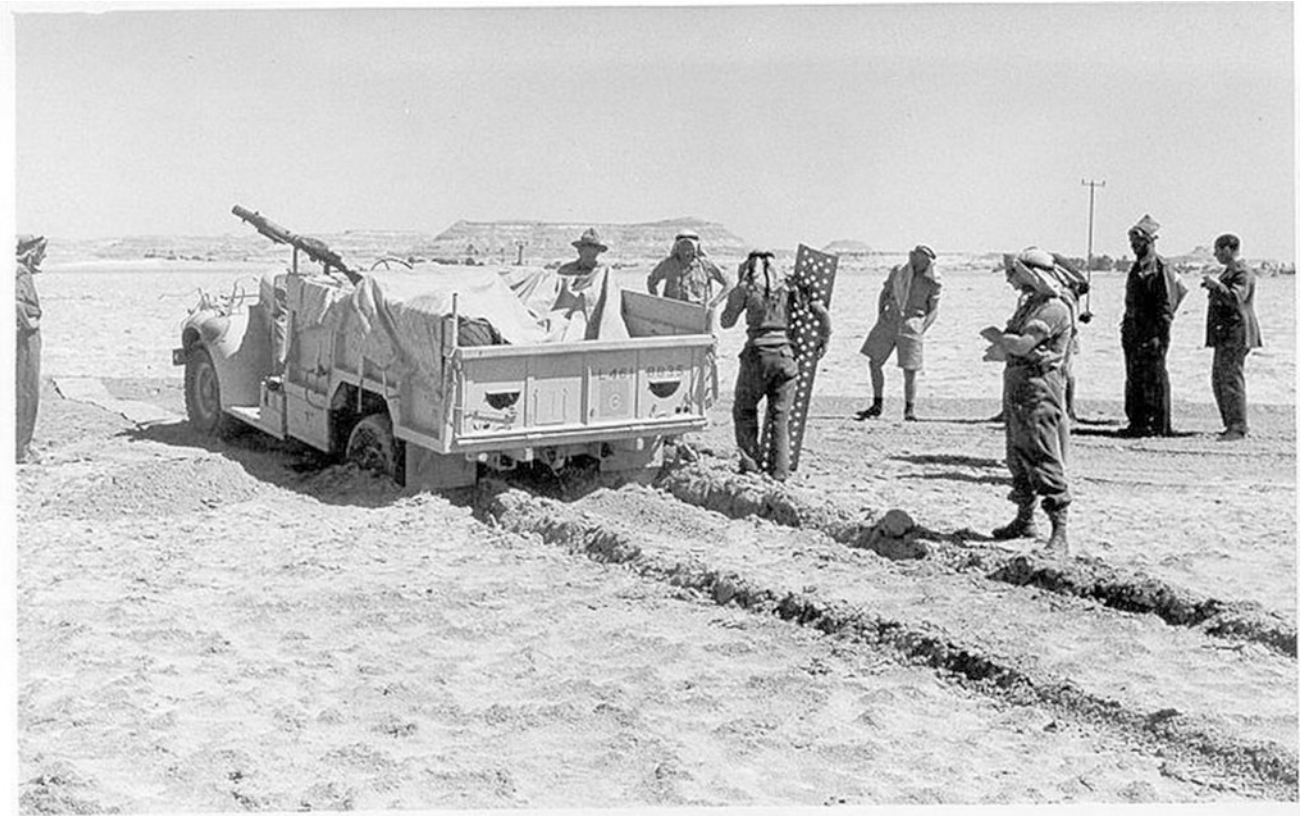
Fig. 22.5 A stuck vehicle of Bagnold's Long Range Desert Group being prepared to unditch. Mats have been laid in front of the front wheels and a sand channel is about to be pushed under the right rear
