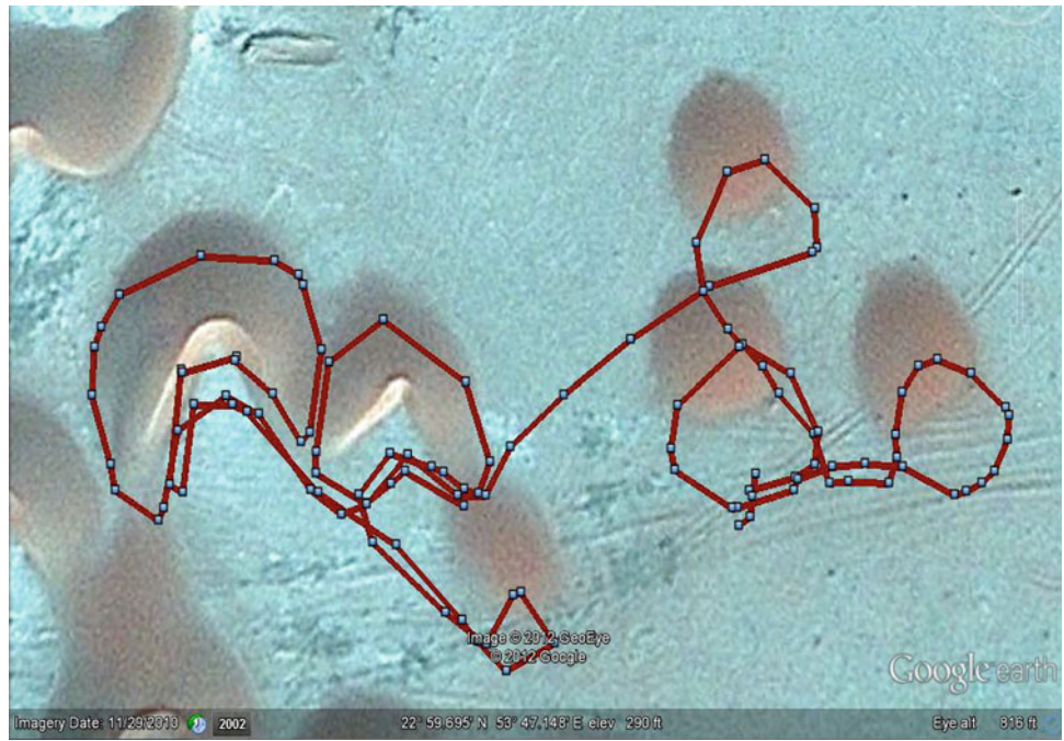
Fig. 9.5 A GPS track obtained simply by carrying an ordinary handheld receiver while walking the perimeter and slip faces of four dome and two barchan dunes south of Liwa in the United Arab Emirates. The track was made in December 2012, while the satellite image was obtained in November 2010. The smallest dunes have moved some 10–14 m, while the barchans have moved by 6–8 m. Image generated with Google Earth, with data from Lorenz and Radebaugh
