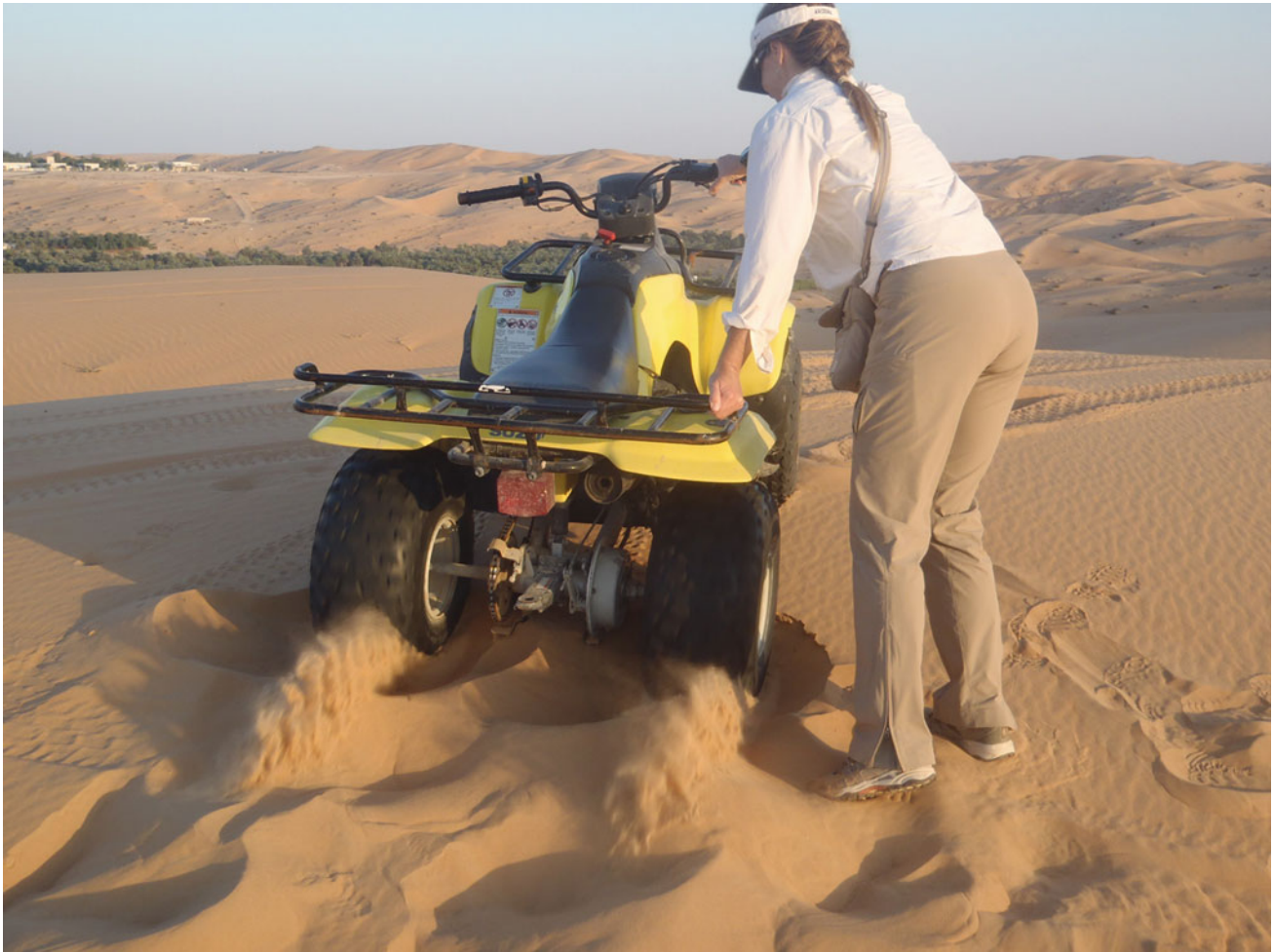
Fig. 22.9 Dismounting (and even, as here, pulling up on the back of the bike) will reduce the wheel loading and thus offer a better chance that the sand under the wheels will hold without failing. Photo R. Lorenz
