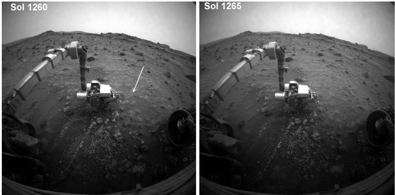
Fig. 16.15 Rapid aeolian change on Mars: a timelapse pair of images taken by the Spirit rover on Mars, five days apart. These images are analyzed in Sullivan et al. (2008) to determine a \sim 2 cm ripple
