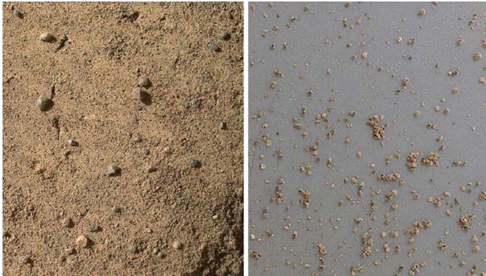
Fig. 12.23 Close-up view of Martian soil with the Mars Hand Lens Imager MAHLI. At left is the surface of the ‘Rocknest’ sand shadow, while at right is a sample of sieved sand ( <150\ \mu\text{m} ) from the interior of the feature. Image PIA16570. NASA/JPL-Caltech/MSSS
