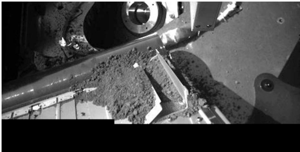
Fig. 16.22 An image from the robotic arm camera on the Phoenix lander, having dumped Martian regolith onto the sample hopper of a Thermal and Evolved Gas Analyzer (TEGA) instrument. One of the two doors (about 2 cm wide and 8 cm long) is only partially open, and
