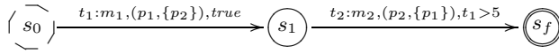
Fig. 7. A business protocol which may stall in state s_1 when the participant p_2 decides not to generate the message m_2
