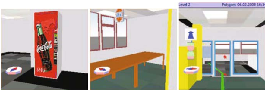
Fig. 15 (left, middle) Detailed objects like soda dispensers and tables can act as landmarks. (right) HYBNAVI’s view while navigating a user
