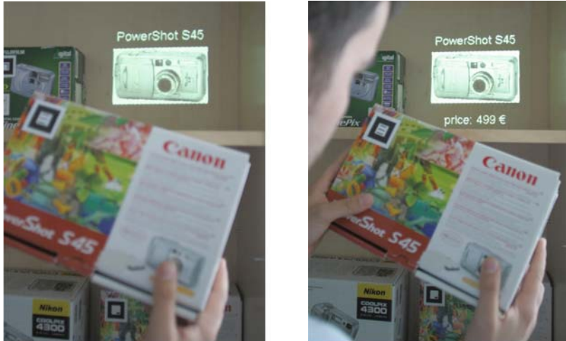
(a) Initial display showing a picture of the product and its name (b) Price information displayed on a PAD as an answer to the user's request
