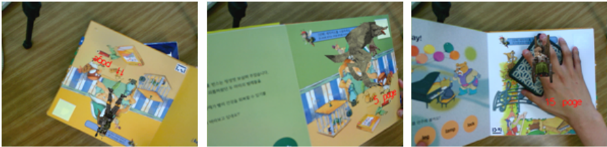
Fig. 4. Pose estimation under ( left and middle ) viewpoint changes, ( right ) serious occlusion
