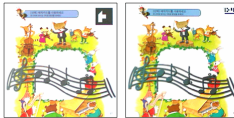
Fig. 2. (left) a page with a traditional fiducial marker, (right) a page with our page marker
