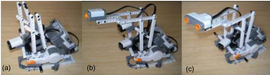
Fig. 3. Reconfiguring a curious robot limb. (a) Lower limb and compass sensor (b) Jointed arm with touch sensor and accelerometer (c) Jointed neck with ultrasonic distance sensor.
