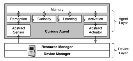
Fig. 1. Architecture for a curious, reconfigurable robot using the Lego Mindstorms platform
