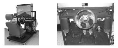
**Fig. 2.** The *AdRacer* driving simulator, together with steering wheel, stereo speaker, foot pedals, eye-tracking camera (*above steering wheel*) and infrared emitter (*above speakers*)
