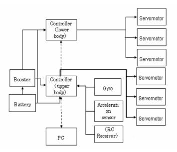
Fig. 5. Hardware construction of centaur robot
