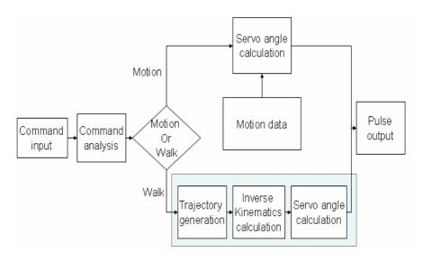
Fig. 3. Software construction of humanoid robot
