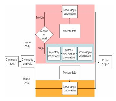
Fig. 6. Software construction of centaur robot
