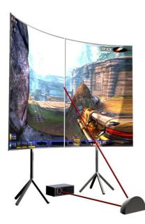
Fig. 1. Drawing of our prototype surround display, 110° horizontal FOV
