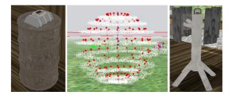
Fig. 1. Threats (left) are simulated as omni-directional particle emitters (middle), and sensors are simulated as particle detectors (right)
