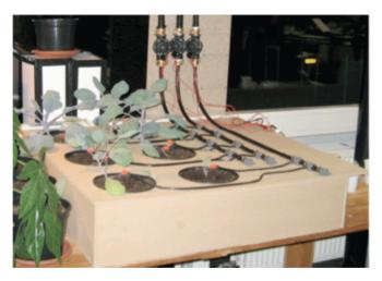
Fig. 9. Health display system (the valves are visible in the back of the installation and the dripping system is visible above each pot)
