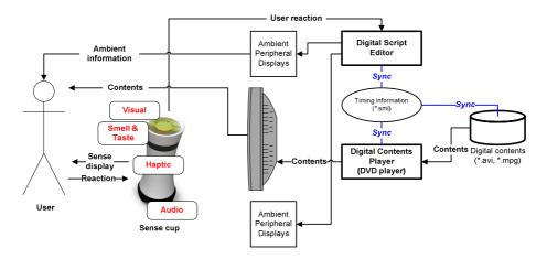
Fig. 5. Configuration of overall Sense cup system
