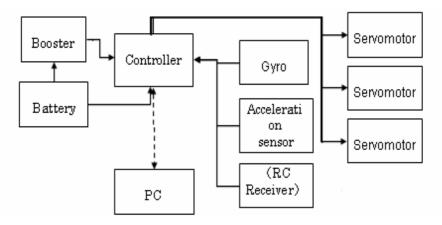
Fig. 2. Hardware construction of humanoid robot
