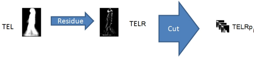
Fig. 4. Generating high frequency residual low resolution test patches
