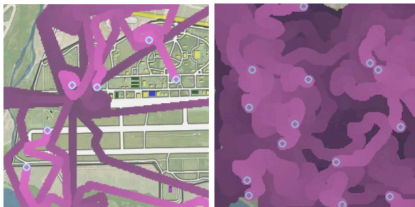
Fig. 2. Base patrolled by a set of UAVs dropping a visit pheromone: initial exploration phase (left) and stabilized phase (right). Brighter color means more pheromone.
