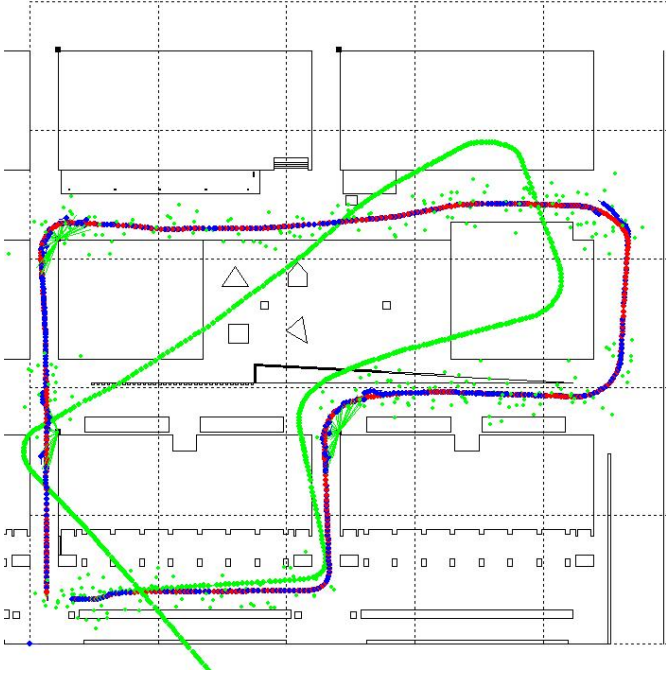
Fig. 6. Simulation of a position tracking experiment. Red poses are for ground truth. Blue poses are the output of the filter. Green poses form the odometry path. Little green dots are GPS data. Green segments are camera detections.
