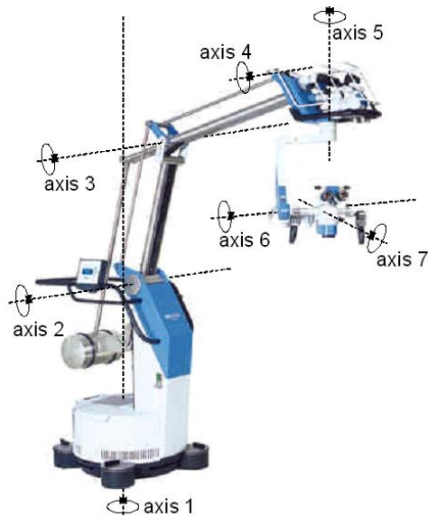
Fig. 1. HI-R 1000 microscope and the tripod FS4-20 with its six motorised axes (1-3 and 5-7) are presented. An additional joint (4) at the end of the parallelogram-arm compensates rotations of axes 2 and 3 and keeps axis 5 parallel to axis 1.
