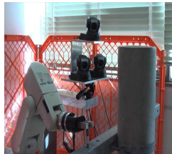
(e) Insert the bolt into the hole using the force control
