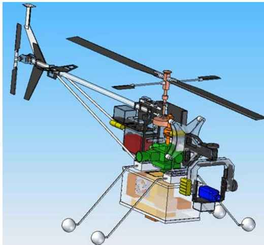
Fig. 6. A view of the CAD model of Bergen Twin Observer; the transparencies allow to see hidden parts, e.g., avionic box and fuel
