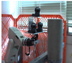
(b) Move the bolt to a place which is 2 cm above the hole
