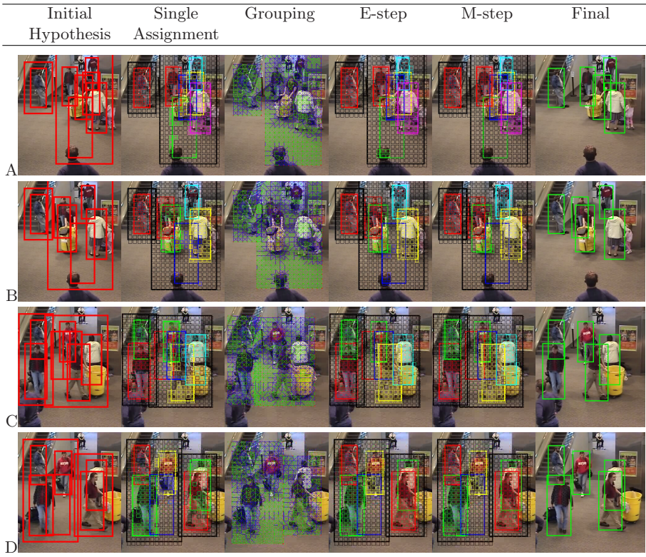
Fig. 4. Six stages of the crowd segmentation process are illustrated for four test images. Overlapping patches of 0.5W are used. However, for clarity smaller patches are shown. The initial hypotheses generated by the head and shoulder classifier are shown in the first column. In the second column, the patches are shown color coded based on their strongest direct assignment as calculated by the whole body classifier. The null hypothesis is shown in black. In the third column, neighboring patches with strong similarity measures based on color constancy are connected by green line segments. The assignment of patches to hypotheses based on the first E-step is shown in the fourth column. The assignment after multiple rounds of both the E and M steps are shown in the fifth column. The final segmentation is shown in the last column.
