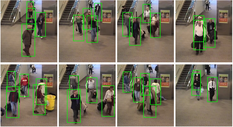
Fig. 5. This figure shows an assortment of crowd segmentation results. Note that the algorithm produces the correct segmentation in case of severe partial occlusion (right column), and in presence of cleaning equipment (bottom left) and a variety of suitcases and bags.
