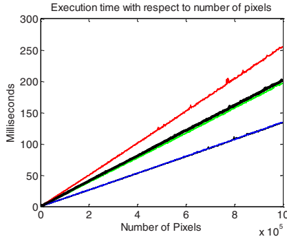
Fig. 9. Execution time as a function of image size on square images ranging from one pixel to one mega-pixel. Curves are shown, from fastest to slowest: for a blank image and an image filled with ramps (blue and black, almost identical), a pixel-size checkerboard pattern (thin green line), natural image (thick black line) and a random image (thin red line). Note the completely linear timings, which include both passes.
