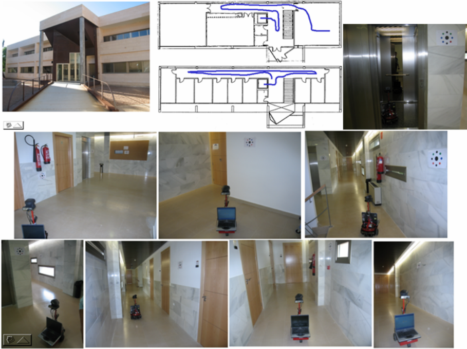
Fig. 4. Above: Building and paths of the robot in the first and second floor. Below: Different locations of the robot in the route and patterns founded.
