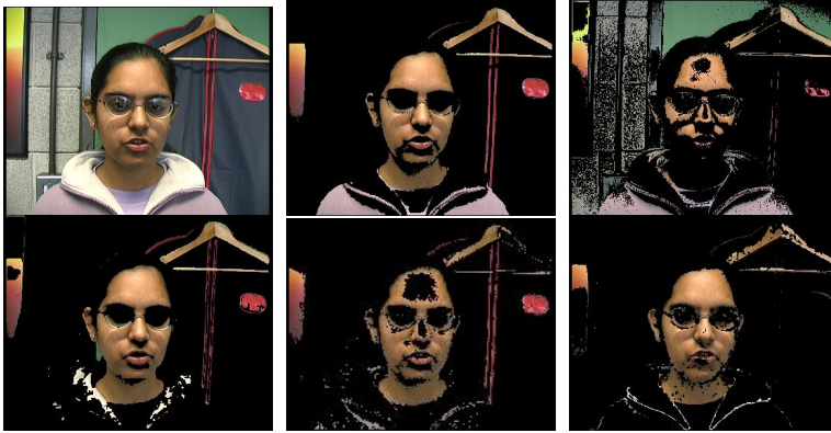
Fig. 6. Results from the VALID database with a complex background. From left to right, top to bottom: original image; results for explicit RGB rules; results for SPM in RGB, T = 0.15 ; results for SPM in HSV, T = 0.05 ; results for SPM in YCbCr, T = 0.03 ; results for our model.
