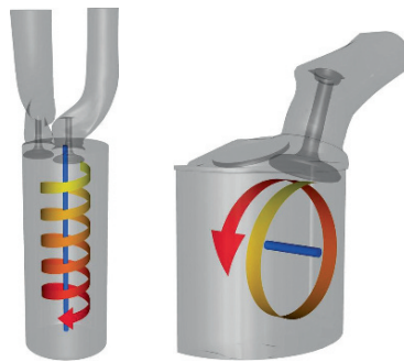
Fig. 3. (left) The swirl motion of flow in the combustion chamber of a diesel engine. Swirl is used to describe circulation about the axis aligned with the valve cylinder. The intake ports at the top provide the tangential component of the flow necessary for swirl. The data set consists of 776,000 unstructured, adaptive resolution grid cells. (right) Some in-cylinder flows require a tumble motion flow pattern in order to mix fuel with oxygen. Tumble flow circulates around an axis perpendicular to the cylinder axis, orthogonal to the case of swirl motion
