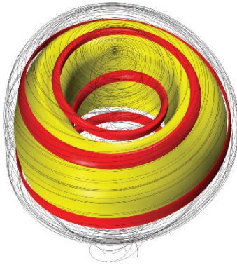
Fig. 5. Primary (yellow) and secondary (red) islands rendered as stream surfaces
