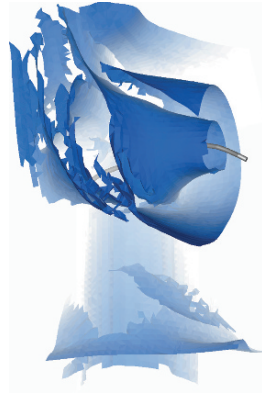
Fig. 5. Steady positive-time FTLE ridges (blue) around vortex core line (gray tube) in front of the Francis divider
