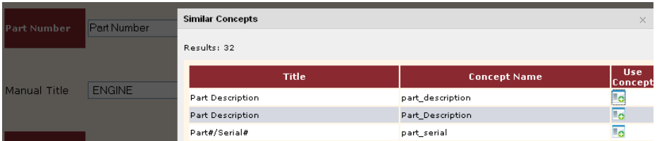
Fig. 3. K-Forms: search and reuse of similar concepts before creating new ones (here search for concepts similar to part_description is shown)
