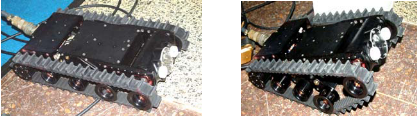
Fig. 1. Polymorphic tracked robot in its down position (left), partly raised position (right)
