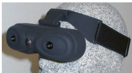
Fig. 8. Video see-through HMD “AR-vision-3D”
