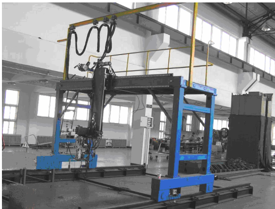
Fig. 5. The mechanisms of welding robot
