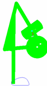
Fig. 1. The six-bar linkage modeled in Pro/E. The thin line is the track of the toe.
