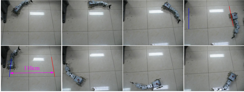
Fig. 9. The circular motion achieved by body-deformation steering. The anticlockwise snapshots show the different moving positions in a circle successively. The blue and red lines in two captures denote the same locations in the actual ground.
