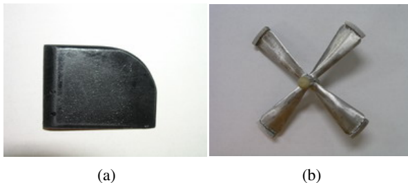
Fig. 2. The alternative flipper and wheel-paddle. (a) The flipper driving the robot “crawl” on land. (b) The wheel-paddle with a heterotypic structure, acting as the primary driving mode on land.
