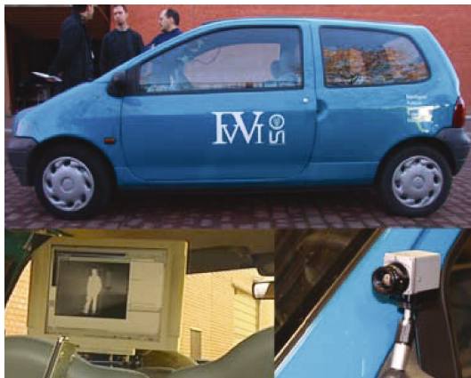
Fig. 1. (top) IVVI: Intelligent Vehicle based on Visual Information. ; (bottom-left) Vehicle's screen; (bottom-right) Infrared camera.
