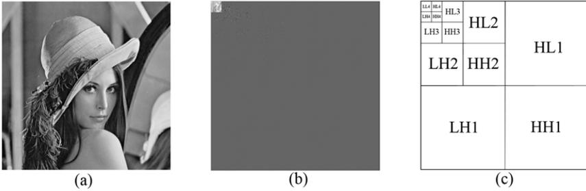
**Fig. 2.** (a)  $512 \times 512$  Lena image, (b) decomposed Lena after applying 4-levels of 2D DWT, (c) convention of (b)
