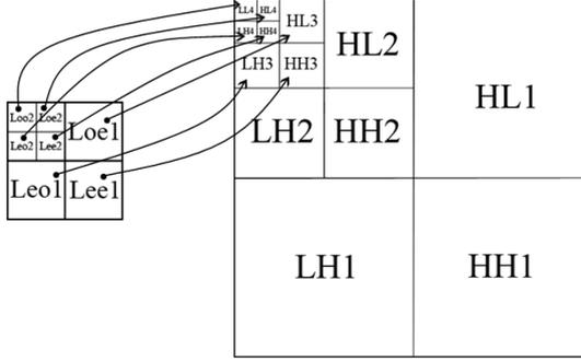
**Fig. 4.** Corresponding subbands in the reconstructed logo and the wavelet decomposed image
