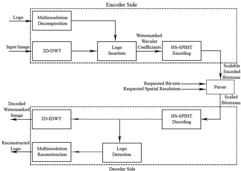
Fig. 1. Block diagram of the proposed system
