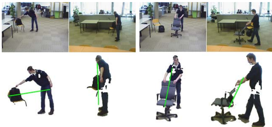
Fig. 4. Typical images from a sequence where objects are used; Top view: input images, bottom view: segmented objects. Left: a bag is carried and put down ( \bar{\phi} = 80.8^\circ , \bar{\rho} = 21.3 ); right: a chair is used as a walking tool ( \bar{\phi} = 24.6^\circ , \bar{\rho} = 8.5 ). The main axis is drawn in green.
