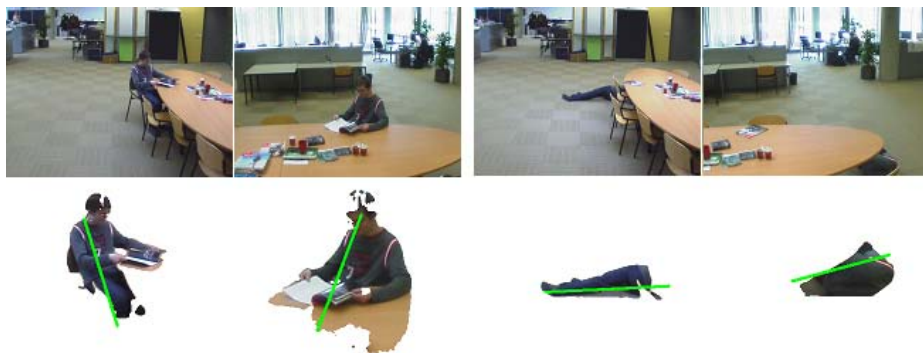
Fig. 5. Typical images from sequences where occlusions occur; Top view: input images, bottom view: segmented objects. Left: a person is reading and is partially occluded for both cameras ( \bar{\phi} = 21.19^\circ , \bar{\rho} = 5 ); right: a person has fallen and is occluded partially for both cameras ( \bar{\phi}_{max} = 87.7^\circ , \bar{\rho} = 0.3 , the fall is detected). The main axis is drawn in green.
