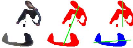
Fig. 6. Example of a bad segmentation result; the middle of the person is not detected. Left: foreground mask; middle: result when both blobs are seen as one object; right: result when both blobs are seen as separate objects. The main axis is drawn in green.
