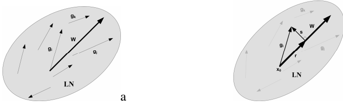
Fig. 3. The idea behind the structural tensor is to represent a local neighbourhood LN with a single orientation vector \mathbf{w} , which is accurate if most of the gradients in LN coincide with \mathbf{w} (a). This can be checked by minimizing a cumulative sum of the residual vectors \mathbf{s} in LN (b).
