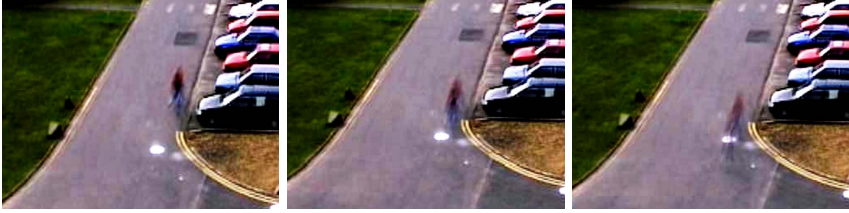
Fig. 1. Simulated long exposure images in a typical surveillance environment (crops of larger images, contrast-stretched). As the exposure time increases (from left to right: 1, 2 and 3 seconds), the moving subject appears more and more blurred and transparent.
