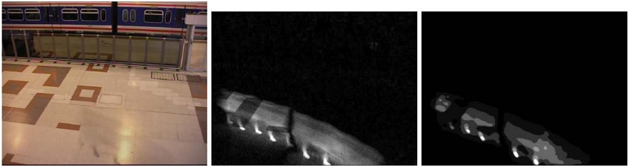
Fig. 6. A person walking in a public building (synthesized from video): 4 seconds exposure. Note that feet are highly visible in the difference image as they are fixed for longer periods of time. Also note that patterns in the background influence the difference image as they affect contrast to foreground.
