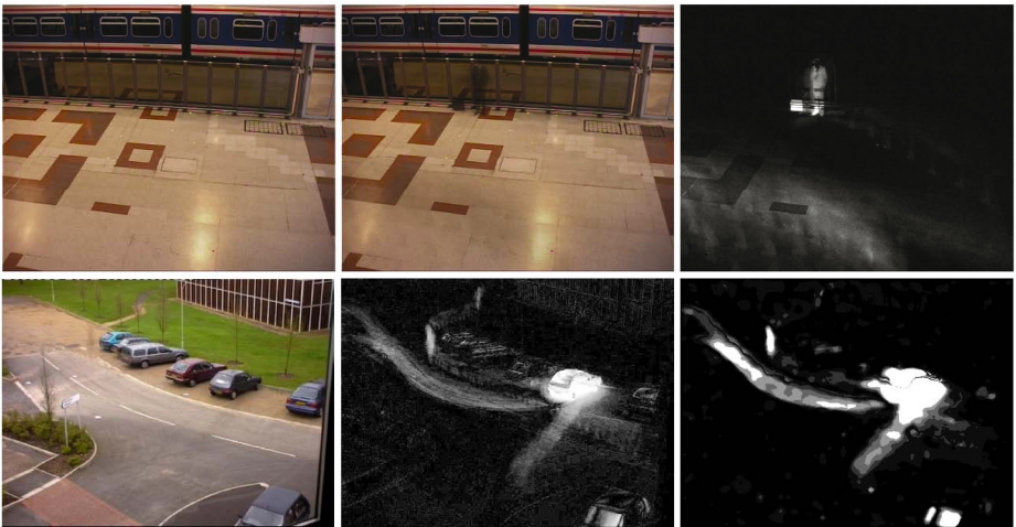
Fig. 9. Up : 15 seconds exposure; note path of person and its clear silhouette where he stood still; his image is also visible, semitransparent, in the long-exposure frame. Down : 5 seconds exposure; note path of car while parking, and trace of nearby motion. Images synthesized from public videos[1].
