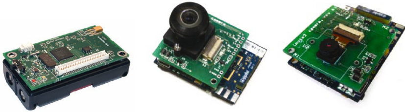
Fig. 2. Nodes of wireless sensor networks and wireless camera networks, battery powered. Only a very careful use of their limited computational and communication resources can allow them to reach a years-long lifetime.
