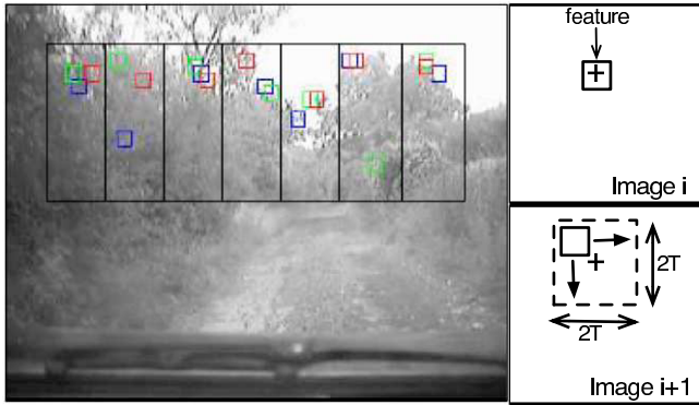
Fig. 1. Stabilization algorithm: Feature detection step (left) and pattern matching step (right)
