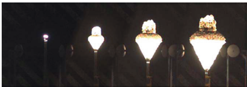
Fig. 3.18. Detonation propagation in mixture of H-2 aluminum (3- \mu m-diameter particles) in a 64-mm-id tube with NM + 10% TEA (mixture 65% aluminum by weight). Time between frames, 50 \mu s. The distance between the detonation front and the luminous particle cloud of about 6.5 cm corresponds to a reaction onset time of about 15 \mu s
