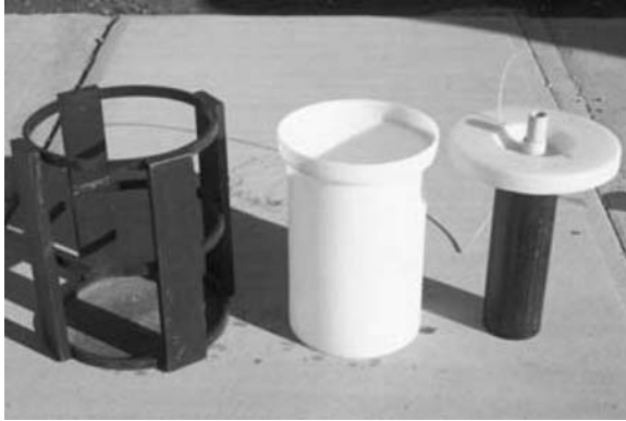
Fig. 1.38. FAE III device tested by Murray et al. [106]; vortex-generating cage ( left ) and chamber with initiator fluid surrounding burster charge ( right )
