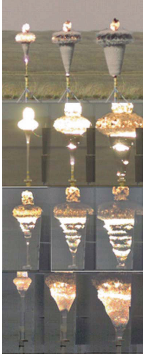
Fig. 3.16. Ignition regimes for cylindrical charges containing sensitized NM and aluminum particles. Conditions from top to bottom : subcritical case for the dispersion of H-95 particles ( 114 \pm 40 \mu\text{m} ) in a 19 mm inner diameter (id) tube, 114 \mu\text{s} between frames; critical case for H-15 particles ( 20 \pm 10 \mu\text{m} ) in a 48.5 mm id tube, 86 \mu\text{s} between frames; critical case for H-50 particles ( 54 \pm 21 \mu\text{m} ) in a 34 mm id tube, 57 \mu\text{s} between frames; supercritical case for H-50 particles in a 74 mm id tube, 80 \mu\text{s} between frames
