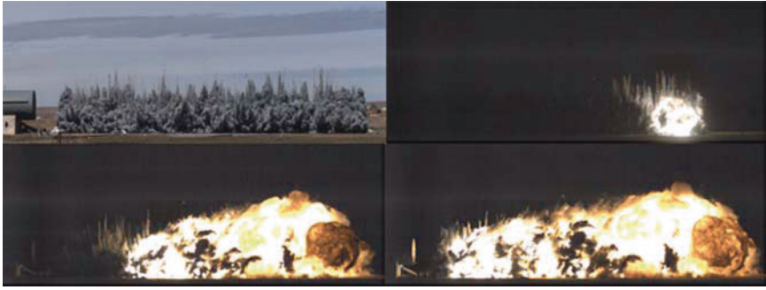
Fig. 2.22. DDT in an unconfined 3\text{ m} \times 3\text{ m} \times 18\text{ m} flaked aluminum–air cloud. Top left: Aluminum suspension. Top right: 8 kg C4 explosive initiation. Bottom left and bottom right: Detonation propagation [22]
