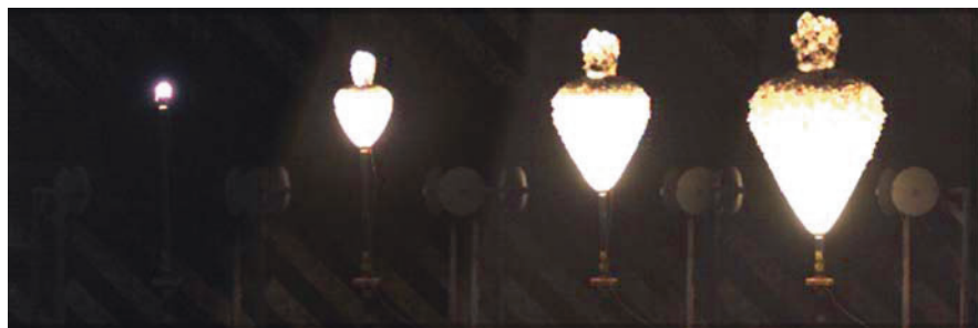
Fig. 3.17. Detonation propagation in a mixture of Alex aluminum (100–200-nm-diameter particles) in a 41-mm-id tube with NM + 10% TEA (mixture 25% aluminum by weight). Time between frames, 50 \mu s. The distance between the detonation front and the luminous particle cloud of about 2.6 cm corresponds to a delay time for particle reaction of about 6 \mu s
