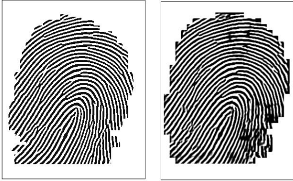
Fig. 7. Examples of fingerprint image after filtration using proposed algorithm (left image) and Gabor filtering (right image)
