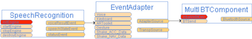
Fig. 10. OI component pipeline that defines the selection of an object by using speech
