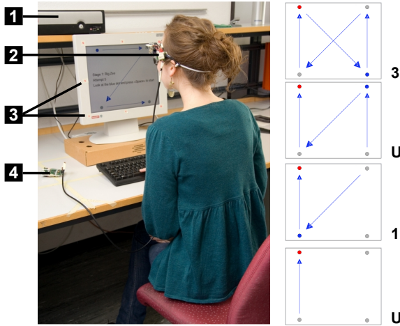
Fig. 3. Experimental setup consisting of a desktop computer running the game (1), the Goggles (2), a flat screen with red dots used for calibration (3) and the Pocket (4). The screenshots on the right show the sequence of eye movements and the generated event symbols for gesture 3U1U (from top to bottom). The red dot denotes the start of the gesture and the blue dot its end point. Blue arrows indicate the order and the direction of each expected eye movement.
