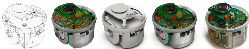
Fig. 2. Development steps for the creation of the e-puck model. Left to right: wireframe of the model; texture map; radiosity map; texture and radiosity maps combined; photo of the real robot.
