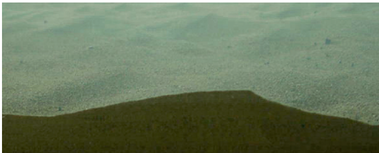
Fig. 6.3. The cross-section profile of an aeolian sand ripple captured in wind tunnel, the axial wind velocity is 12 \text{ m}\cdot\text{s}^{-1} , the sand is natural dune sand sampled from the Badain Jaran Desert, China, and the size distribution of sand particles is shown in Fig. 4.1 (photo by the author et al. in the multi-function wind tunnel of Lanzhou University)
