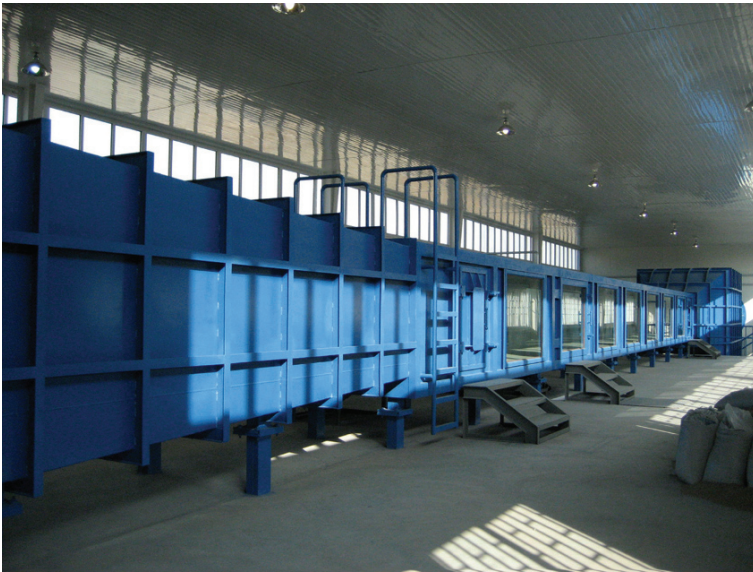
Fig. 2.7. Low-speed blow down wind tunnel (Multi-function environmental wind tunnel of Lanzhou University), which contains four sections: the power part, the rectifier part, the experimental part and the proliferation part. The total length of the wind tunnel is 85 m, the experimental section is up to 20 m, the cross-sectional area is about 1.3 m (width) \times 1.45 m (height), wind velocity is adjustable from 4 \text{ m}\cdot\text{s}^{-1} to 40 \text{ m}\cdot\text{s}^{-1}
