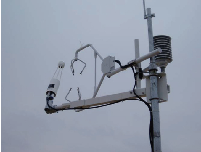
Fig. 2.4. Tower measuring instruments including CSAT3 3-D Sonic Anemometer and LI7500 Open-gas Analyzer (from College of Atmospheric Sciences, Lanzhou University)
