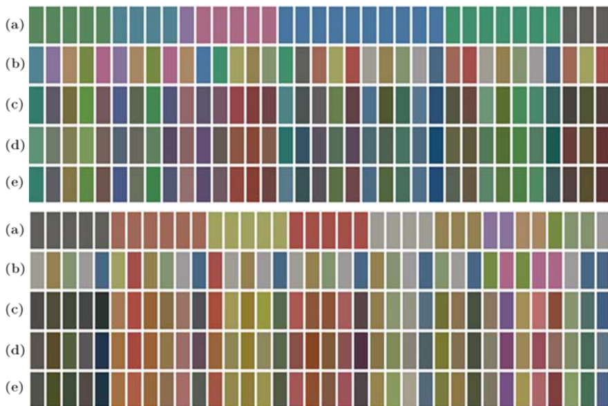
Fig. 6.11. Pigment mixing using our neural network. Row (a) and row (b) are the two source pigments before mixing. Row (c) is the pigment mixing results sampled from real world experiment. Row (d) is the prediction of the pigment mixing behavior using our proposed neural network, but without employing the kernel functions. Row (e) is the prediction using our proposed neural network with the kernel functions
