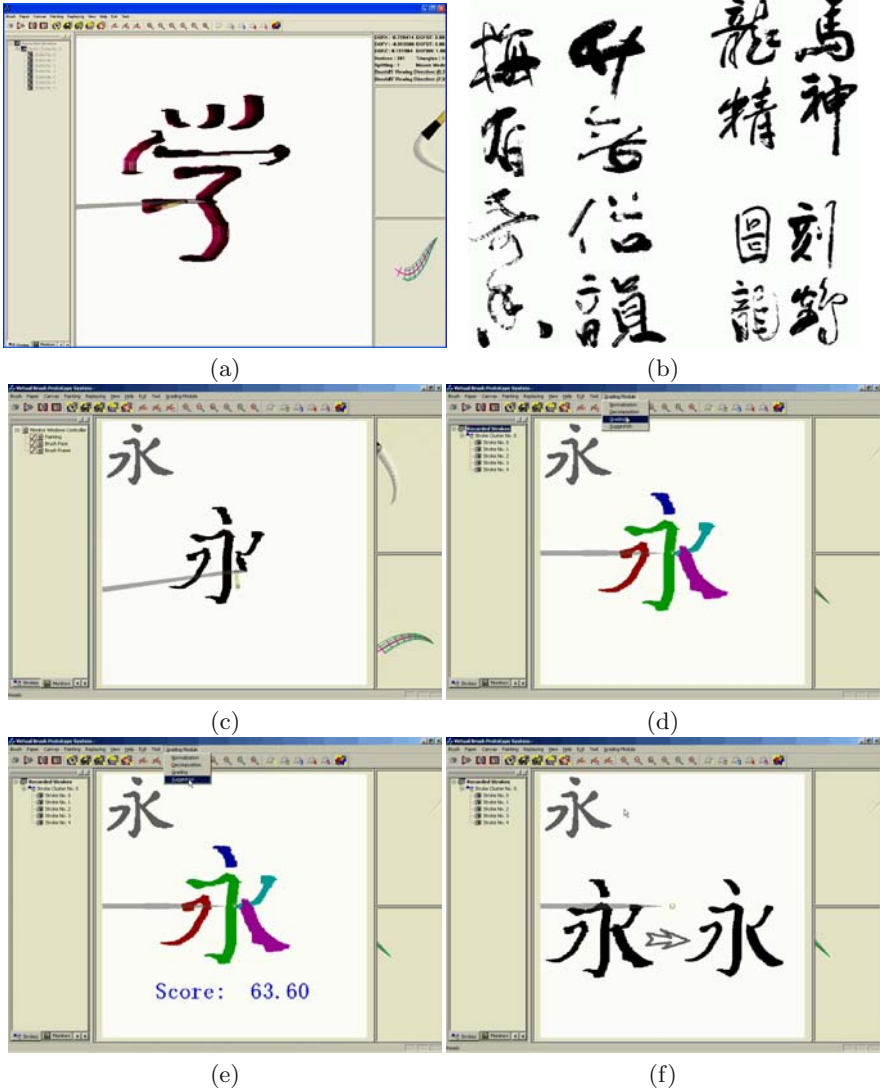
Fig. 10.26. Intelligent calligraphy writing tutoring system: a screen-shot (a), and some calligraphy created interactively using the system (b). (c to f) show a series of screen shots of how the tutoring function works. The user can write a calligraphic character with the virtual brush provided by the system (c). At first the character is decomposed into individual strokes (d). The grading result is given by both the shapes of individual strokes and spatial features of the character (e). According to the scoring, the system can suggest how to improve the writing (f)
