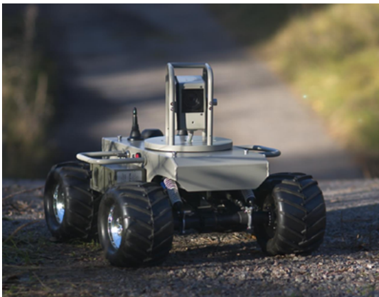
Fig. 1. This Surveillance UGV testbed, developed by SAAB Aerotech, will be used in real-world experiments
