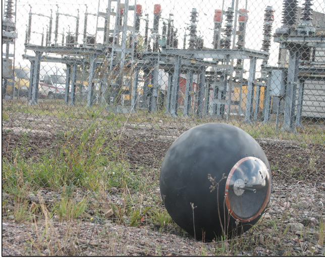
Fig. 1. Groundbot, the Surveillance UGV that will be used in real world experiments ( www.rotundus.se )
