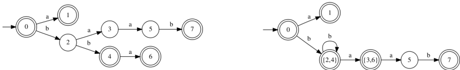
Fig. 3. (left) PTA(S_+) with S_+ = \{\lambda, a, bb, bba, baab\} and \lambda denoting the empty string; (right) a quotient automaton A = PTA/\pi where \pi = \{\{0\}, \{1\}, \{2, 4\}, \{3, 6\}, \{5\}, \{7\}\} . Accepting states are represented as doubly circled nodes.
