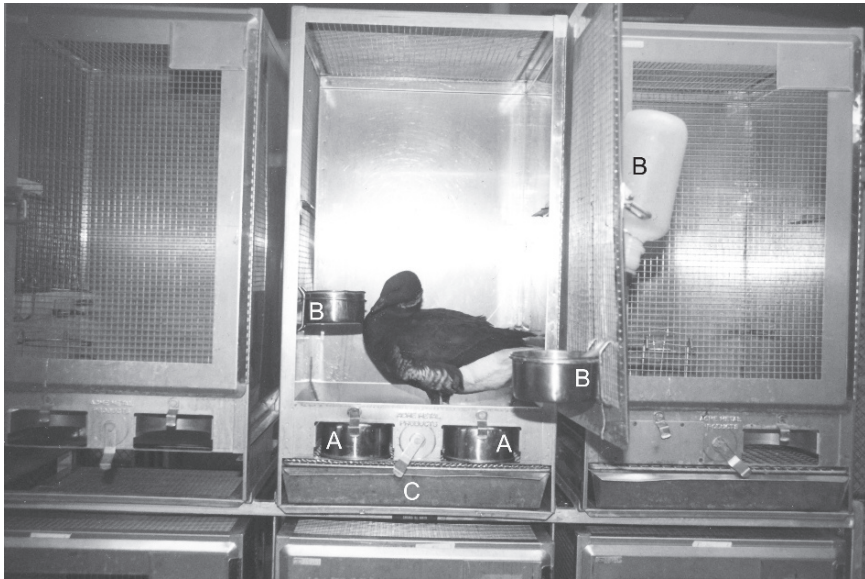
Fig. 4.4 Pacific black brant in a metabolism cage for measurement of food and water ingestion as well as total excretion. Metabolism cages are designed to provide easy access by animals to food (A) and water (B) with minimal spillage during feeding. The cage floor is constructed of mesh that allows excreta to fall through the floor into a pan (C) for collection. Cages for mammals also include screens beneath the floor to separate feces and urine for collection. Mesh on the floor must be large enough to allow excreta to fall through, but small enough to support the animal and minimize damage to the feet. Perches, roosts and nest boxes may be used to provide resting areas within each cage
