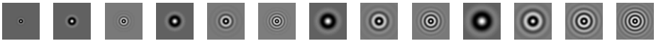
Fig. 5. Schmid filter bank that we use to generate the textons and in turn the histograms
