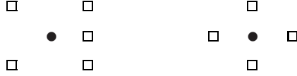
Fig. 2. Two sets of road points that match under Hausdorff distance (for a suitable \epsilon ) even though they should not match in the NRNM problem
