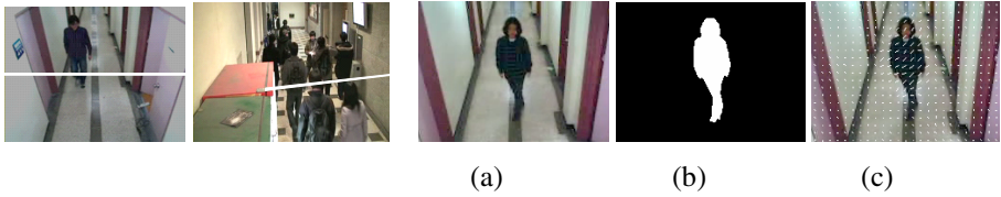
Fig. 1. Examples of virtual gates Fig. 2. Examples of feature extraction: (a) Original image. (b) Foreground image. (c) Motion vectors.
