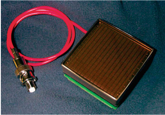
Fig. 10.7 Hamamatsu H8500 flat-panel position-sensitive photomultiplier tube (PSPMT). (From [100]. © 2006 IEEE with permission)
