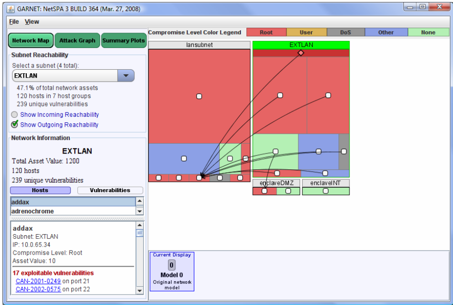
Fig. 2. GARNET in Network Map mode. The arrows indicate outgoing reachability for the EXTLAN subnet.
