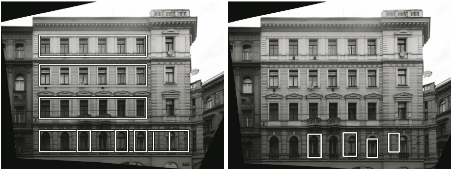
Fig. 3. Left: Hypothesised window-arrays with four additional window hypotheses. Right: Result after restarting the low-level IPM with a hypothesised region of interest.
