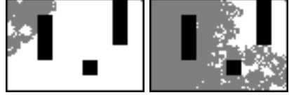
Fig. 7. Explored area when penalty-based reward is used with the negative initialisation of the Q-table and \gamma = 0.99 : after 10^4 iterations in the left part and after 10^6 iterations in the right part of the figure
