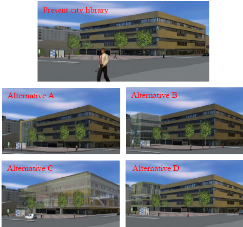
Fig. 1. The VR-model of the actual library and the four suggestions: A, B, and D exploit the place on the left of the actual library and C around and above it
