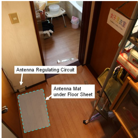
Fig. 6. Deployment of an antenna in front of a restroom (No. 2 antenna in Fig. 4)
