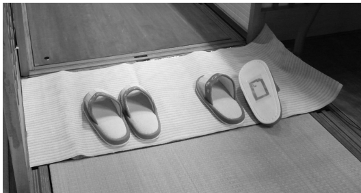
Fig. 2. Slippers with RFID tags (in actual operation, the tags are embedded)
