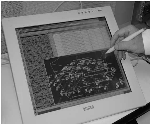
Fig. 3. Pen display GUI showing microarray like quantity data (left) and gene interaction network (lower right)
