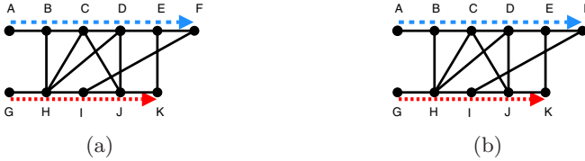
Fig. 1. An instance (G, R, P) of min-DAWN-path containing 2 requests r_1 = (a, f) , r_2 = (g, k) , P(r_1) = (a, b, c, d, e, f) and P(r_2) = (g, h, i, j, k) (sub-fig. a). A valid and conflict-free date assignment and within a minimum number of slots (sub-fig. b).
