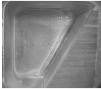
Fig. 2. Oil Flow Picture on Cavity Floor For \frac{L}{D}=2 , M=1.4 no control case and with 30^\circ wedge placed at leading and trailing edge
