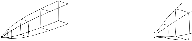
Fig. 1. Geometry of the true streamtraced nozzle. Left: Full view, right: zoom-in view
