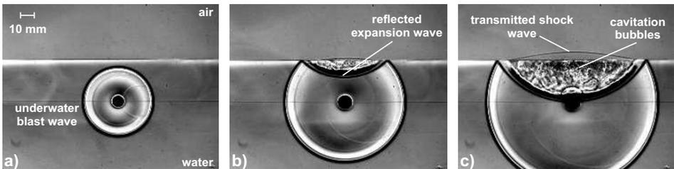
**Fig. 2.** Underwater explosion of 10 mg  $\text{AgN}_3$ . Three frames of a schlieren visualization sequence taken with 500 000 fps, time interval between shown frames  $\Delta t = 14 \mu\text{s}$ .
