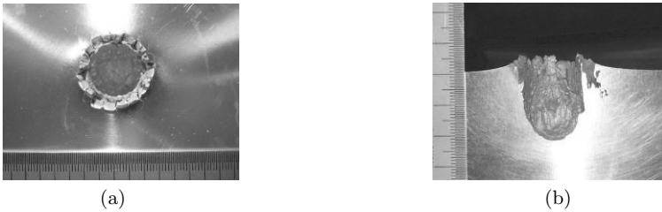
Fig. 7. Target plate after impact (Fe/Al impact (Case 3)): impact velocity = 3.0 km/s; (a) frontal view, and (b) side view of crass section
