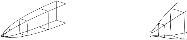
Fig. 1. Geometry of the true streamtraced nozzle. Left: Full view, right: zoom-in view
