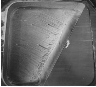
Fig. 4. Oil Flow Picture on Cavity Floor For \frac{L}{D}=6 , M=0.8 no control case and with 30^\circ wedge placed at leading and trailing edge
