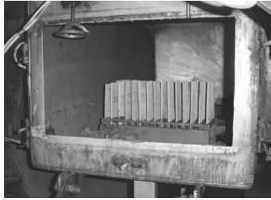
Fig. 3. A photograph of the vatta wood slats mounted inside the shockwave generator for treatment
