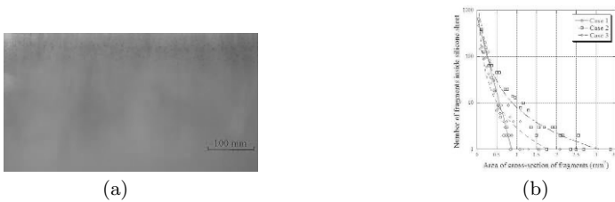
Fig. 8. Captured ejecta fragments inside silicone sheet; (a) sample silicone sheet after HVI experiments (Case 1), and (b) relationship between the size and number of ejecta fragments
