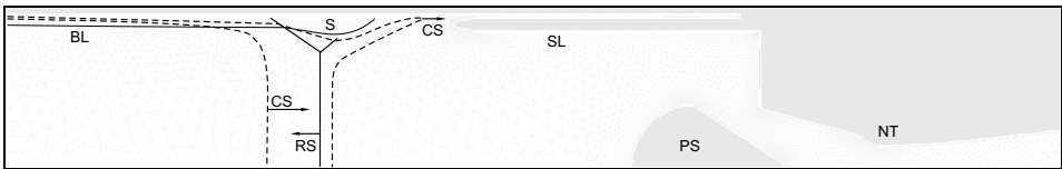
Fig. 2. Sketch of the shock tunnel reservoir region and schematic of the driver gas contamination process. Reflected shock wave (RS), boundary layer (BL), contact surface (CS), separation (S), sleeve (SL), nozzle throat (NT), and particle stopper (PS).
