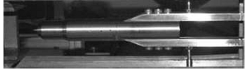
Fig. 2. Inlet Model installed in Wind Tunnel
