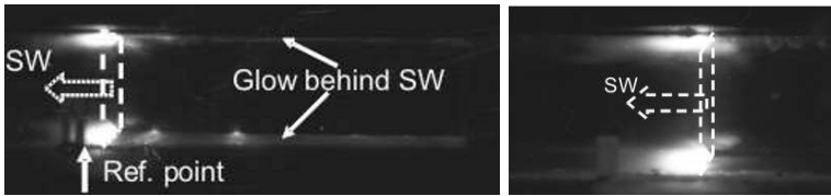
Fig. 2. Left: glow behind SW M = 2 ; x = 9.4 cm; P_0 = 25 torr Right: spatial glow M = 2.6 ; x = 8.5 cm; P_0 = 25 torr
