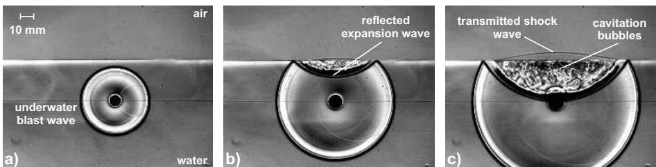
Fig. 2. Underwater explosion of 10 mg \text{AgN}_3 . Three frames of a schlieren visualization sequence taken with 500 000 fps, time interval between shown frames \Delta t = 14 \mu\text{s} .
