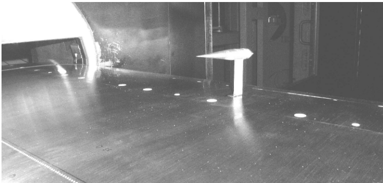
Fig. 3. Transonic wing with conical spike in the DNW-TWG
