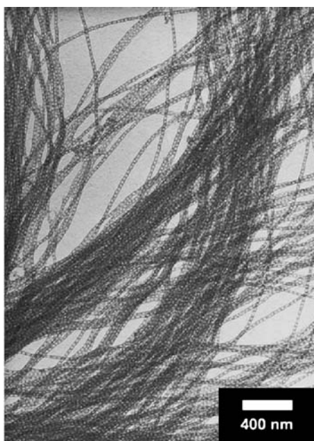
Fig. 23 TEM image of released silica nanowires containing a single row of mesocages obtained with PS(9500)- b -PEO(9500) as the soft template and an AAO hard template ( D_p = 35 nm). Reproduced from [185]. © (2007) Wiley-VCH
