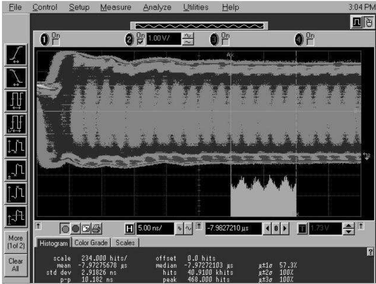
Fig. 8. Histogram of phase distribution in Meta-RO5st digital TRNG. The phase distribution occupies the whole period of the Meta-RO oscillations, significantly increasing the entropy.
